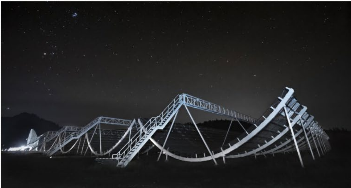
CHIME is an unusual telescope with no moving parts and a huge field of view, which stretches almost from the northern to the southern horizon. (Credit: CHIME)
