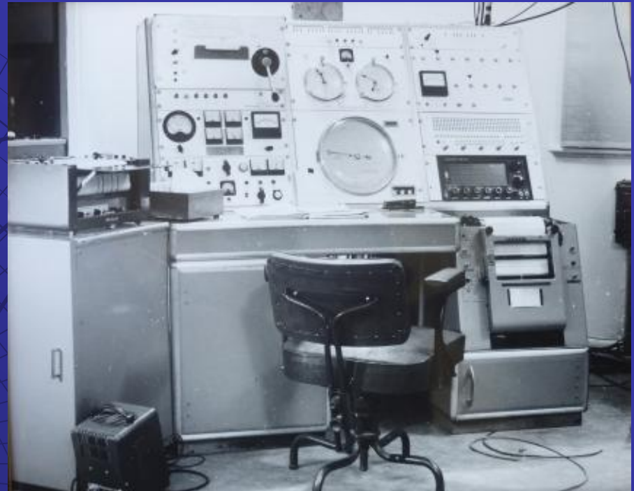
Control desk with on-line monitoring of 11 pencil beams, total power and an immediate contour plot of the zone
